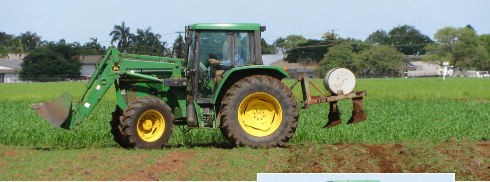
*The Wallace Plough is a five tyned implement designed to break up hard layers in the soil.*
