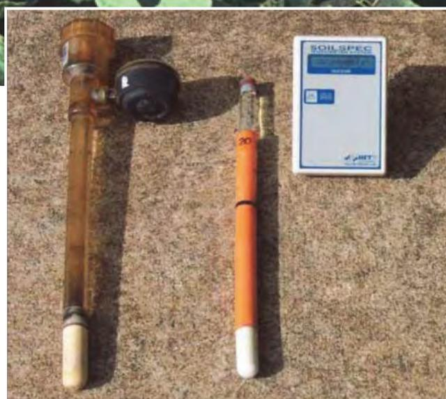
*Two types of tensiometers – the Irrrometer® on the left and the Soil spec® on the right.*
