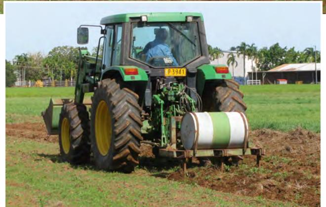
*The weight of the 200 litre drum of water on top of the Wallace plough helps force the rippers into the ground.*
