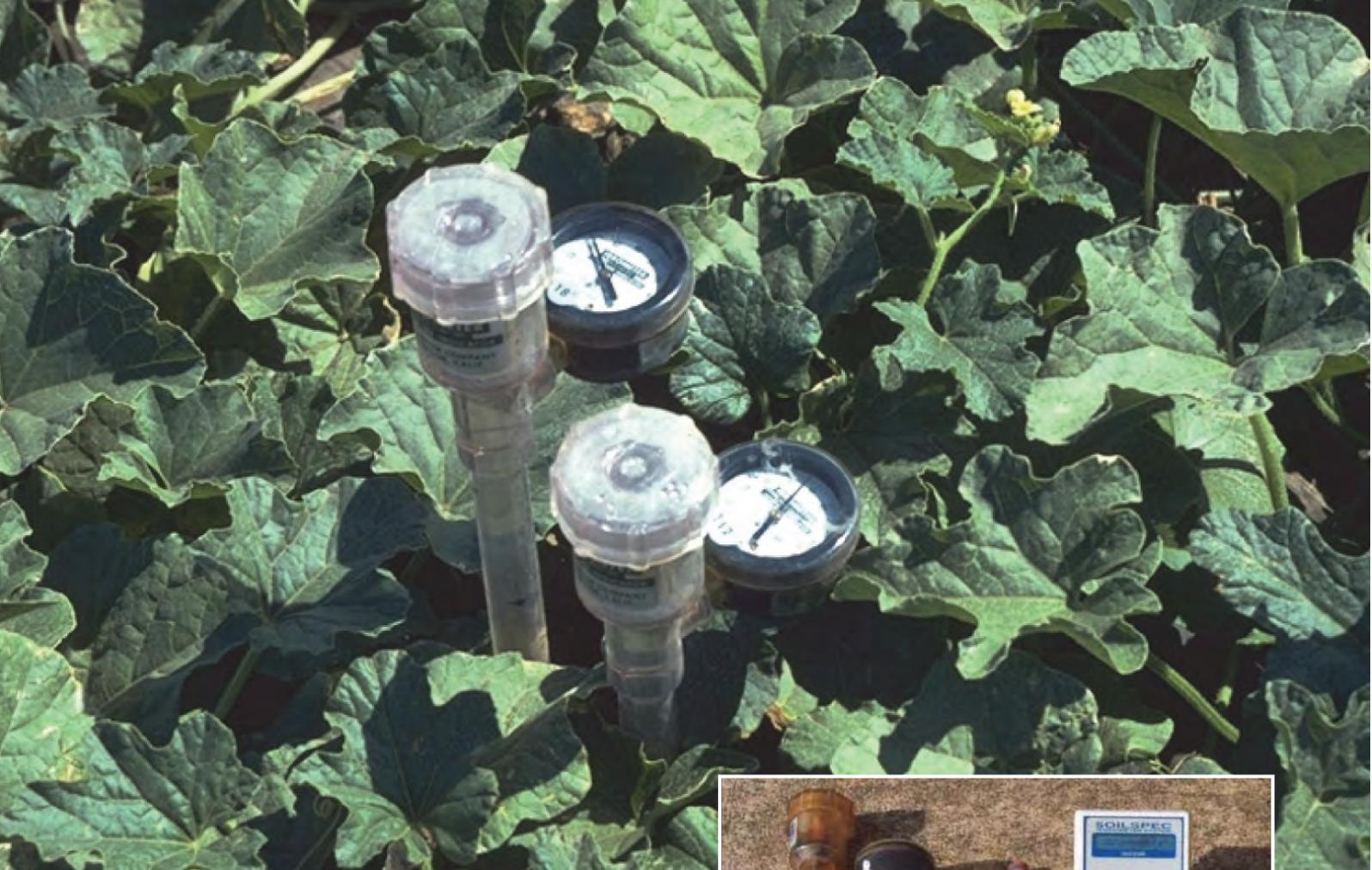
*Tensiometers placed at two different levels in a rockmelon crop.*
