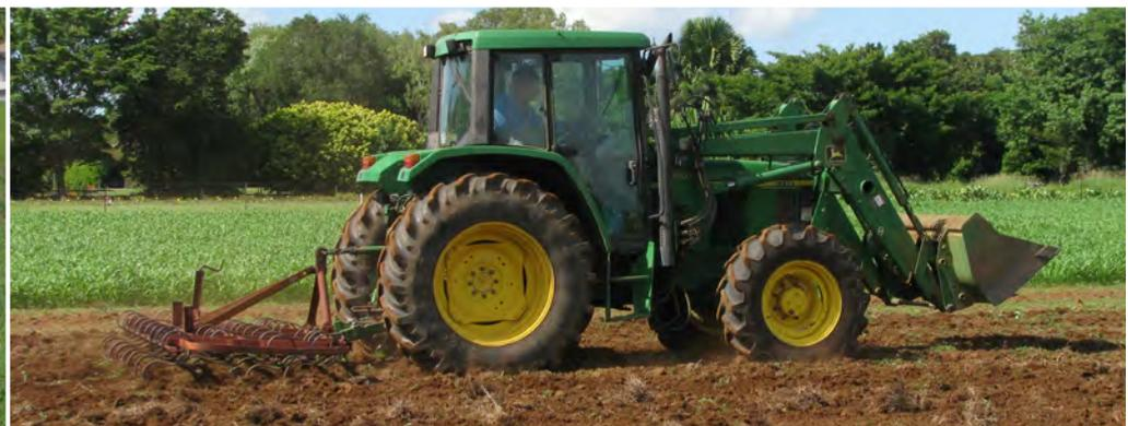
*A spring tyned cultivator is used to work up soil with minimal disturbance.*
